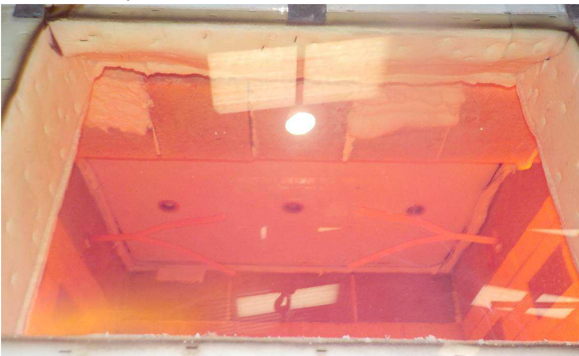
Photo 2.2.2 – Exposed face after 44 minutes.
