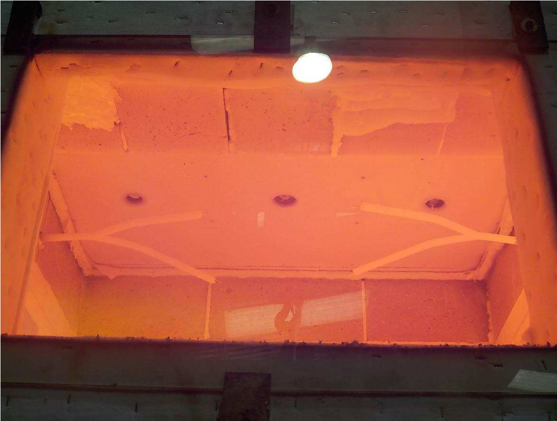
Photo 2.2.3 – Exposed face after 60 minutes.
