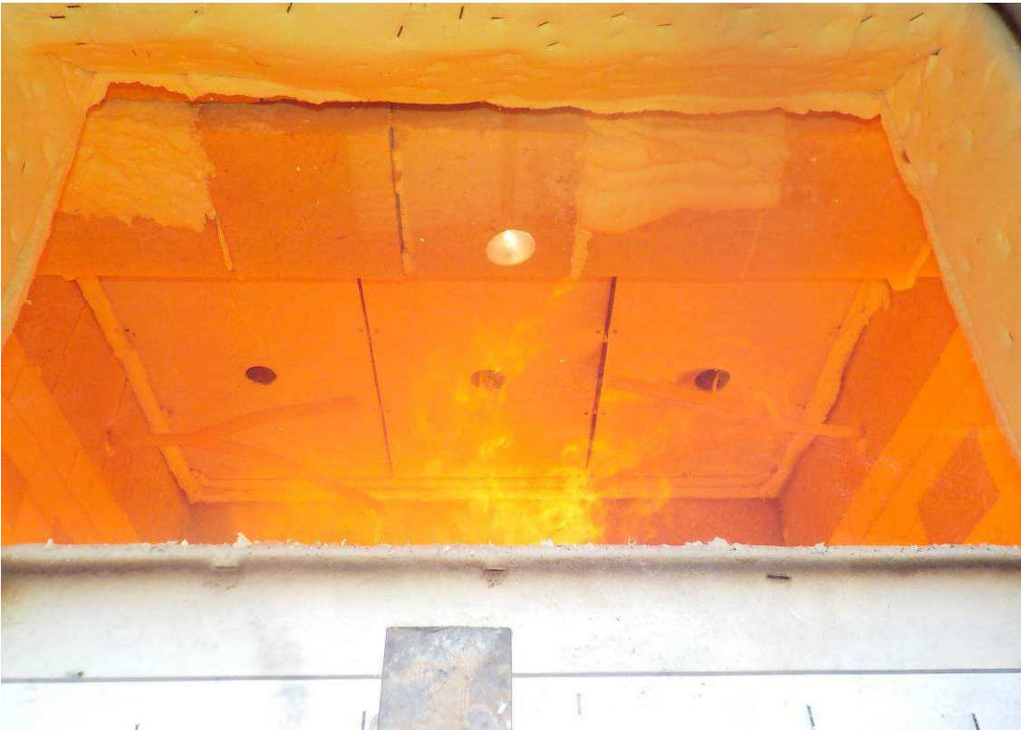
Photo 2.2.7 – Exposed face after 100 minutes.
