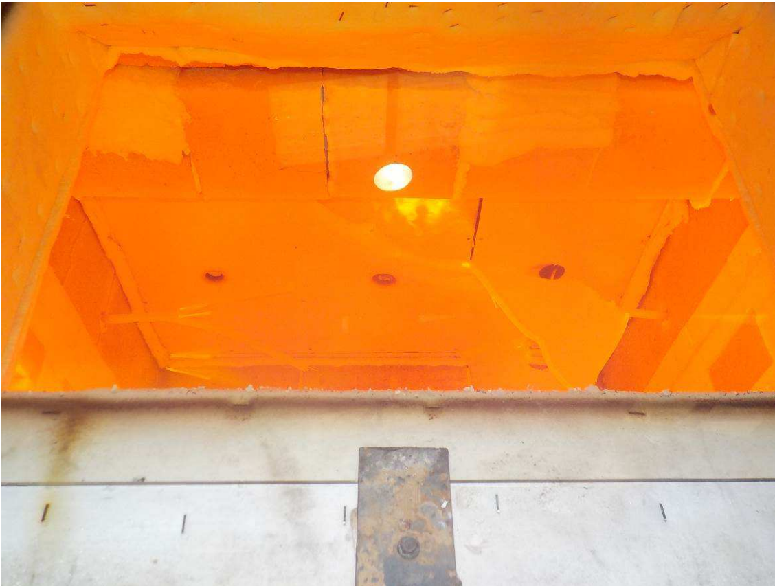
Photo 2.2.5 – Exposed face after 90 minutes.
