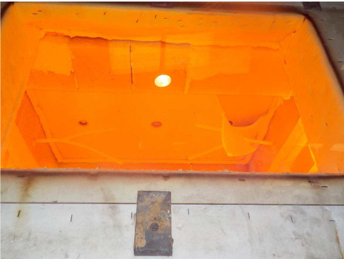
Photo 2.2.4 – Exposed face after 83 minutes.
